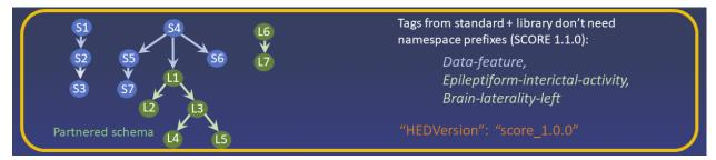
Here the standard schema (blue nodes) and its partnered library schema (green nodes) are merged and viewed as a single schema when the schema is validated and distributed.
